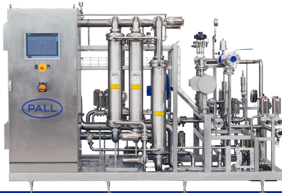
PROFi membrane system for DE-free clarification of beer
