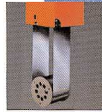
SOP 100-8 with a capacity of 100 l/h oil (SAE 30), belt width 203 mm
