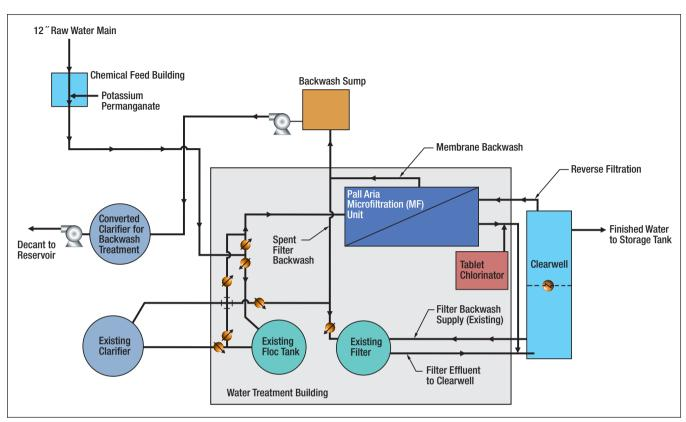
Diagram of Crested Butte's water filtration process.
