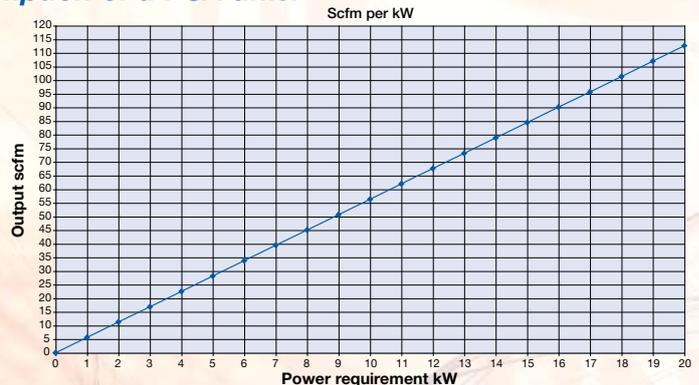
The FLC can be estimated by applying a typical performance index of 4.2 SCFM per brake horsepower (BHP). This equates to 5.63SCFM per kW.
