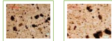
Microscopic examination of contamination found in used fuel filter elements
