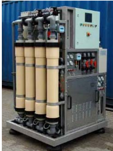
MF pre-treatment upgrade
