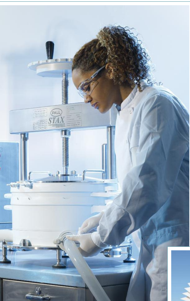
Top: Pilot Scale Chassis with Stax Capsules Right: Seitz Depth Filter Sheet Media
