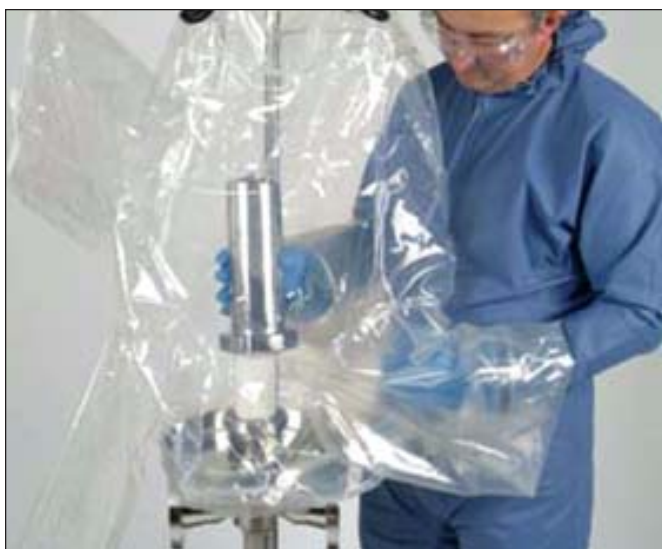
Figure 4. Inserting a new filter into a single cartridge unit using glove bag design.
