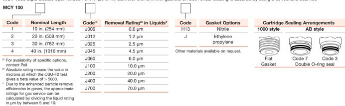
AB style Single open-ended 70 mm (2.75 in.) diameter element with double O-ring at one end
