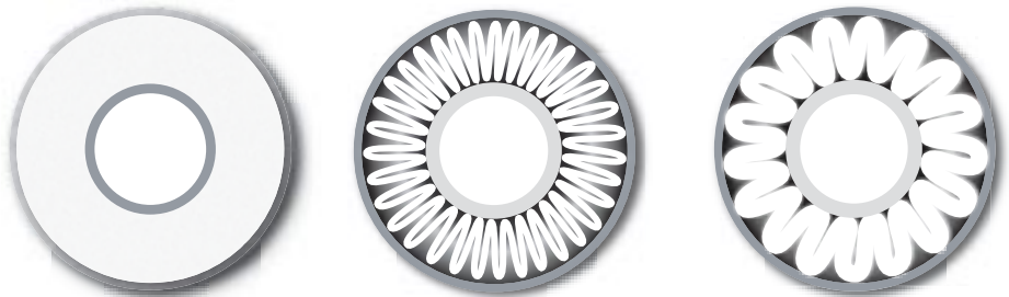
Filter media: Representations of the cross section of three types of depth filter are shown. The image on the left is a cross section of a melt blown cartridge with graded density (tighter pores near the core). The center image is a cross section of a pleated conventional melt blown medium. This cartridge has high area and dirt holding capacity. The image on the right is a cross section of a Profile Star cartridge filter. The media depth, lack of side seal and star pleat structure make it ideal for use as a beer trap filter.
