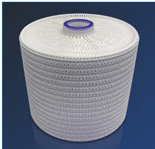
Figure 2: SUPRADisc II modules are robust, cleanable, in-place steamable, and backflushable, satisfying rigorous production requirements in breweries.
