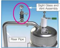
Figure 6a (top) and 6b (bottom): The sight glass and vent assembly, mounted on the feed fluid side of the housing, enables venting of the installation at its highest point, upsteam pressure measurement, and visualization of the feed fluid. The mounting configuration shown in Figure 6a is for 1 to 3-high housings, and the one in Figure 6b is for 4 to 6-high housings.
