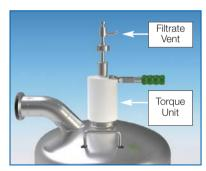
Figure 7: The torque unit is an external tensioning device with preset torque limit, which provides reliable and secure operation without bypass. The filtrate vent, mounted on the torque unit, enables release of air from the filtrate inside the module core.
