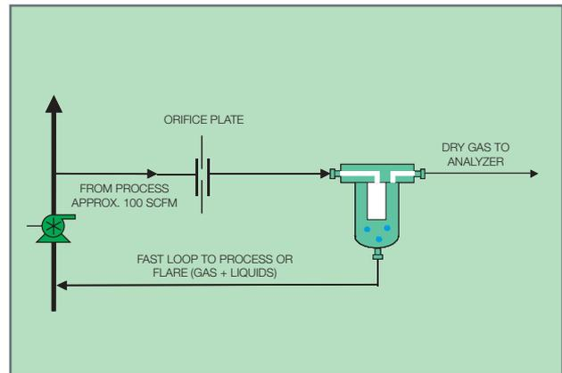
A Canadian refiner was experiencing short filter life and routine fouling of a sulfur in gasoline analyzer. The filter used was a flat sheet hydrophobic membrane about 50 mm (2 inches) in diameter. A Pall Emflon® PF part number MPF4463F002ESTH11 was installed. Analyzer maintenance was dramatically reduced. The Pall filter was removed for inspection by Pall SLS after 11 months of service and was found to be in new condition in terms of degree of plugging and removal efficiency.
