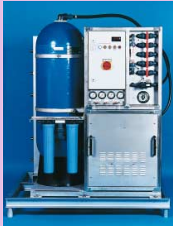
Pall Desalination System
