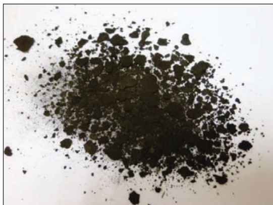
Figure 2: Deposits collected from reboiler tubes at Middle East plant
