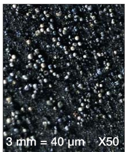
Figure 6: Filter Inlet (Toluene rinsed): Catalyst – 680 ppm Coke –120 ppmw
