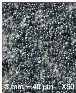
Figure 8: Filter Inlet (Mild H/Cracked Feed): Catalyst – 3500 ppm Coke – 500 ppmw
