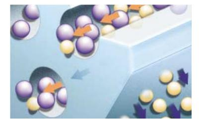
Cross-flow filtration is a continuous process in which the feed stream moves parallel to the membrane filtration surface and purified liquid passes through the membrane. The separation is driven by the pressure difference from one side of the membrane to the other — referred to as transmembrane pressure.
