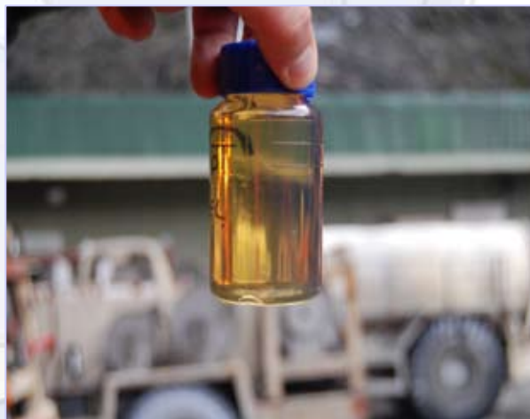
Diesel fuel sample downstream of Pall fuel filters; ISO Cleanliness Code -13/10 and water content below 100ppm
