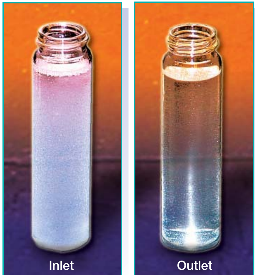
Samples of oil/water emulsion before and after treatment with a Lucid separator
