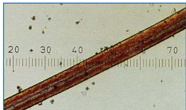
Human hair (75 \mu\text{m} ), particles (10 \mu\text{m} ) at 100x (14 \mu\text{m} /division)
