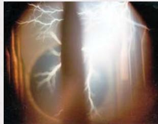
Electrical discharge occurring inside oil tank
