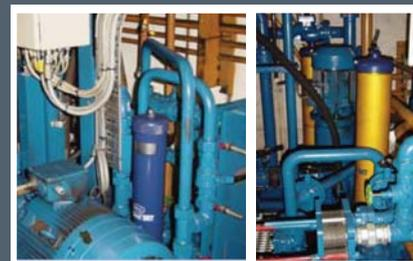
Ultipleat SRT UR319 and UR619 series filters were fitted to the filling and return lines
