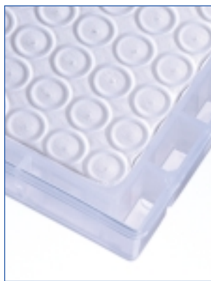
Constructed of two membrane layers – the bottom layer of membrane protects the upstream membrane and acts as a barrier to passive flow.
