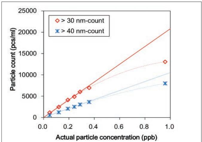
Figure 2. The relationship between the challenge concentration and the particle count. The particle counter is RION KS-19F; > 30 nm and > 40 nm-count are shown.
