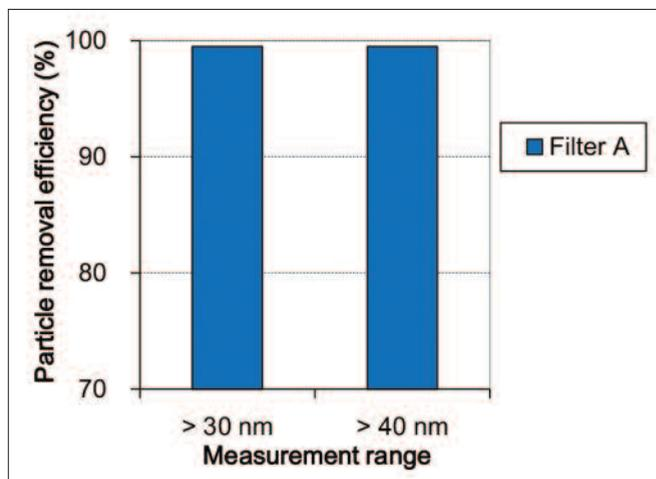
Figure 3. The results of PRE evaluation in 90 °C sulfuric acid using the LPC. PREs were calculated in two different measurement ranges (i.e., > 30 nm and > 40 nm) for each filter. One each of Filter A ~ E was evaluated. The flow rate was 10 L/min for all the filters in this figure.
