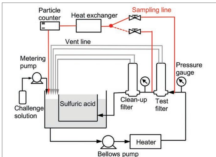
Figure 1. Test line for particle removal efficiency evaluation of filters in high temperature sulfuric acid.
