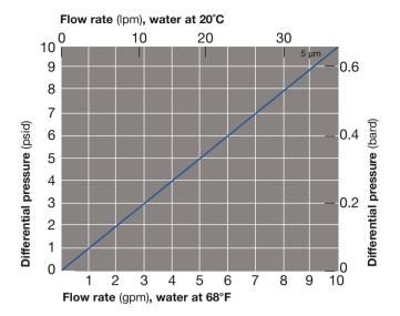
Flow rate is for a 25.4 cm (10 in) cartridge. For liquids other than water, multiply differential pressure by fluid viscosity (cP).
