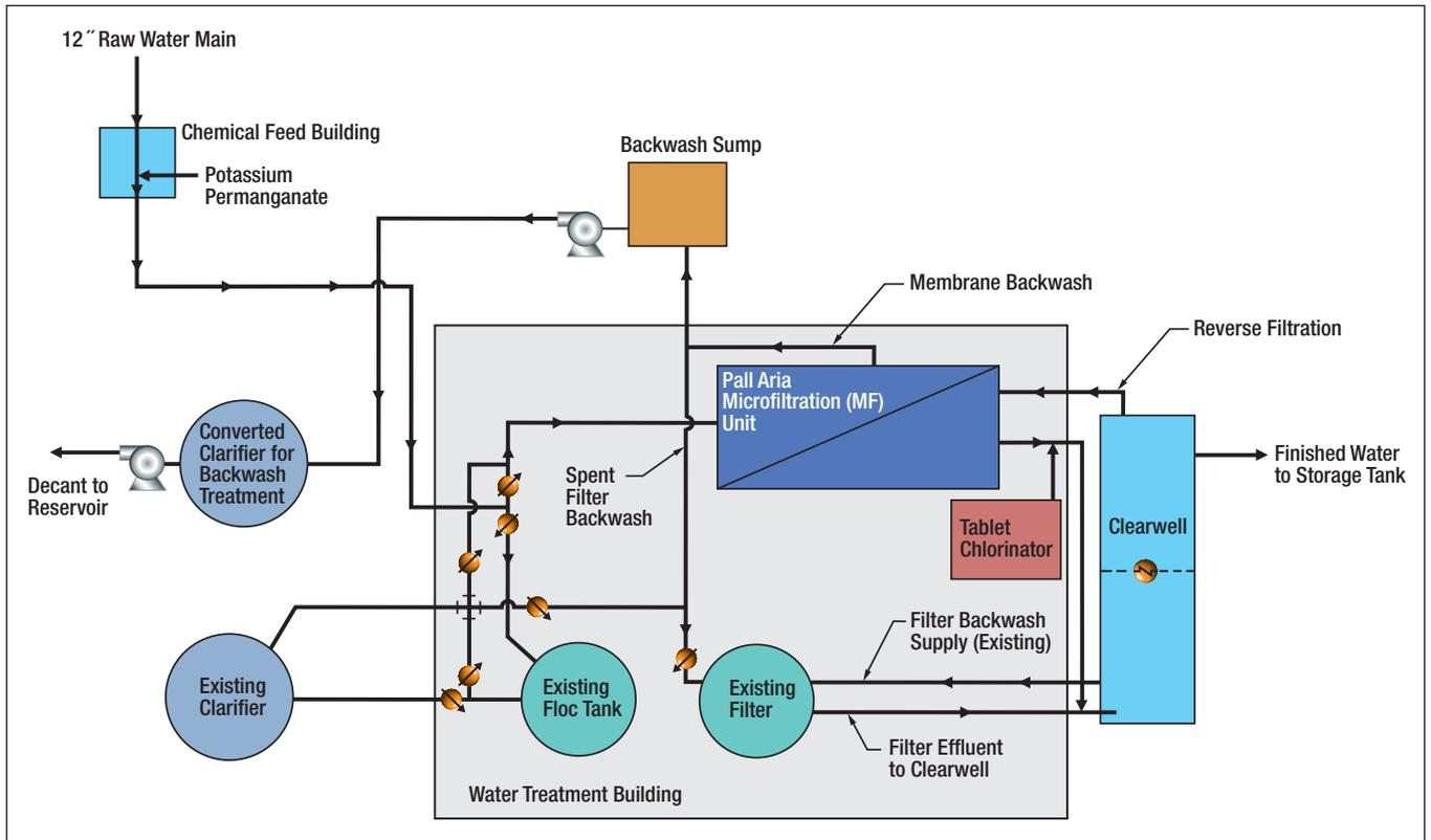
Diagram of Crested Butte's water filtration process.
