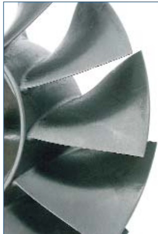
1 Axial compressor: Negligible erosion
