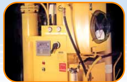
Oil purifier system
