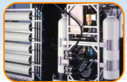
Nanofiltration and reverse osmosis systems
