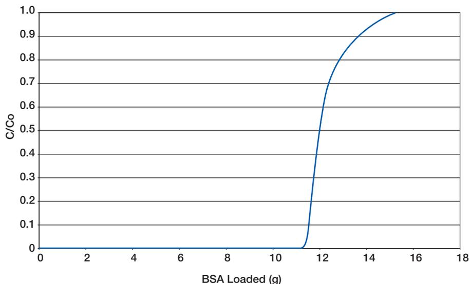
The ratio  $C/C_0$  is the ratio of the BSA concentration in the effluent and in the original feed plotted against the mass of BSA loaded onto the capsule Mustang Q membrane. Initial breakthrough occurs after 11.6 g of BSA has been loaded.
