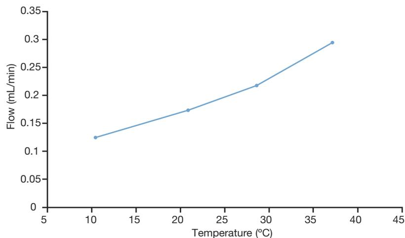
In order to achieve a stable temperature, during the WIT, the water temperature used for WIT should be adjusted to the temperature of the room. If the water supply does not allow such a temperature control and adjustment, the water should be decanted into a container (carboy or similar) and left in the room in which the WIT is to be conducted so that the water temperature can equilibrate to the temperature of the room before testing commences.
