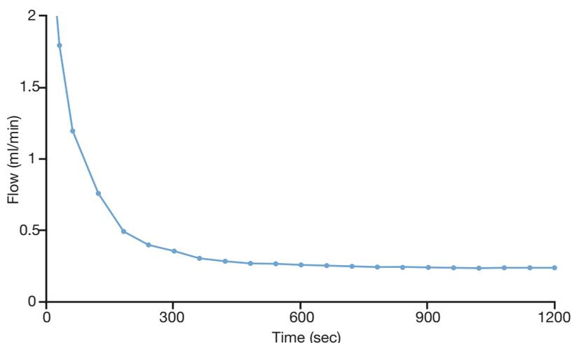
All of the parameters mentioned have been shown to be time dependent (see Figure 4) such that the initial flow rate drops quickly (within 5 minutes) as the pleats compress, and the other factors exert less and less of an effect, until a plateau is reached which is due to evaporative loss of water through the membrane.
