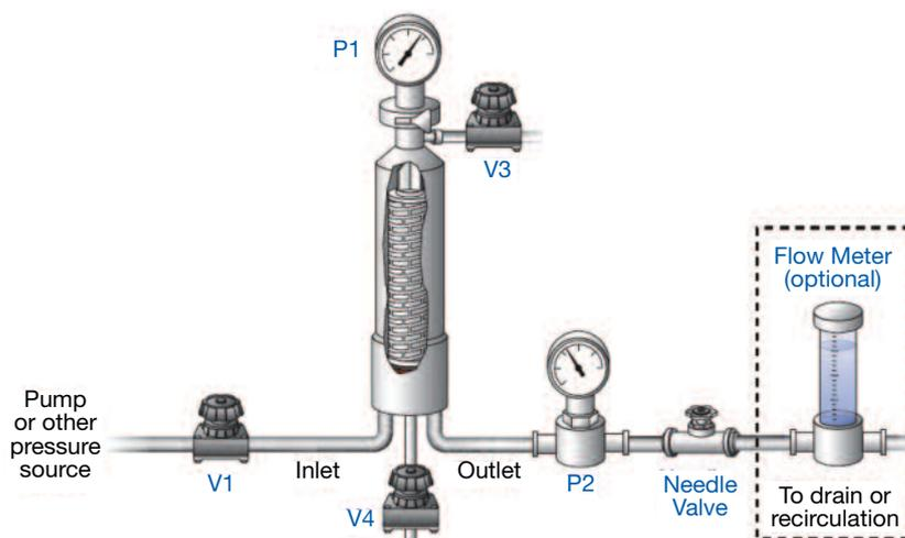
The filter cartridge must be completely covered with water and be in an upright position as shown in Figure 3 to prevent air bypass through any membrane which is uncovered, leading to falsely high WIT values.
