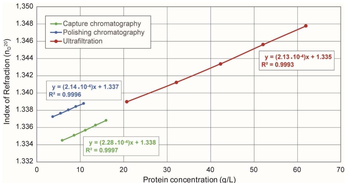
Strong linearity, as seen in the determination coefficients in Figure 1 of these standard curves for all ranges of concentrations (from ~4 to more than 60 g/L) confirms that concentration can be calculated in real time directly from the signal of the mPath IoR monitor.
