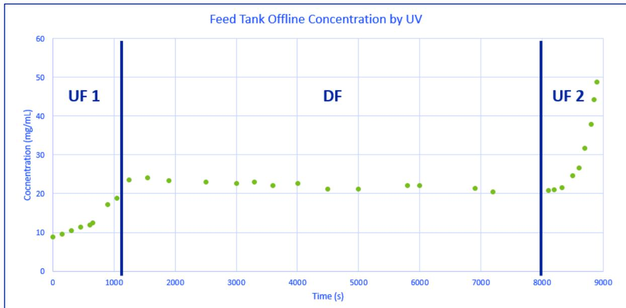
Figure 2 demonstrates the feed tank concentration profile during the experiment. There is an increase in concentration during both ultrafiltration steps and whereas a stable profile is seen during diafiltration. This profile is typical of UF/DF/UF. The signals obtained by the mPath IoR sensor for all three streams were analyzed and are shown in Figure 3.
