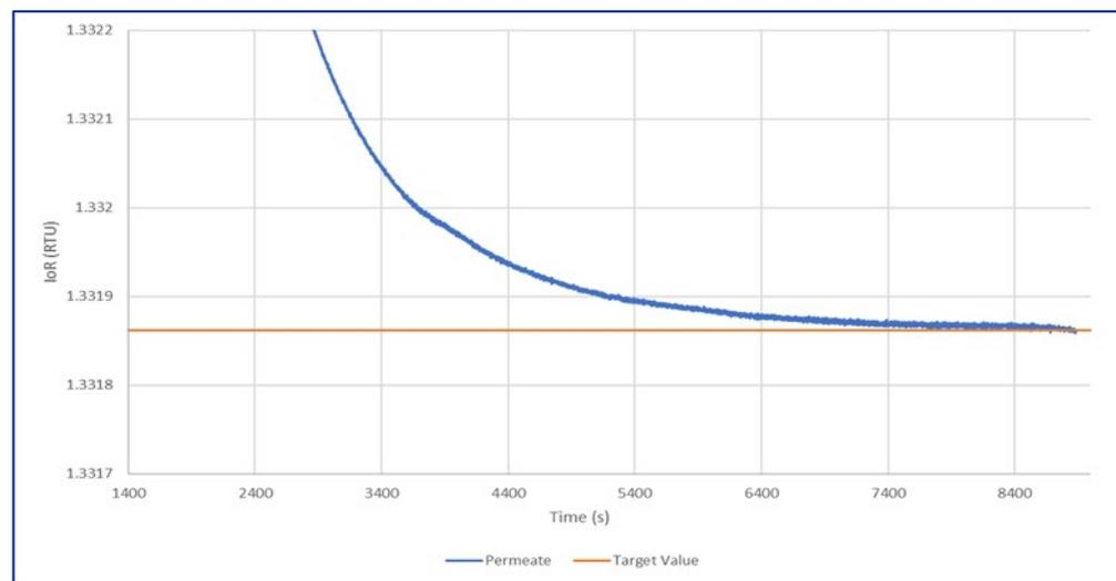
It is shown that the permeate stream will reach an asymptotic value when buffer exchange is completed. The index of refraction (IoR) value of the desired final formulation buffer can be obtained beforehand to define a set target value. This is shown to be a straightforward approach to identifying the completion of buffer exchange in real time. Ultimately buffer use is minimized, and overall process times are reduced.
