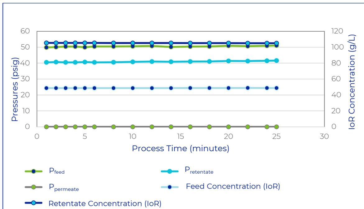
The data shown above demonstrates that the mPath IoR can be used to monitor process stability during SPTFF. The IoR signal can also be used to indicate fouling of the membrane as well and any other process deviations. This allows for fast detection of undesirable process changes.
