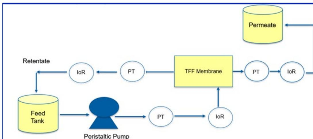
High concentrations are commonly obtained during UF/DF/UF. Consequently, an inline UV sensor is not effective for concentration monitoring due to signal linearity limitations. Thus, it is common practice to obtain process samples to then measure offline with UV. In the figure below (Figure 2) we show the offline concentration measurements of the feed tank throughout the experiment. This is then used to compare against the concentration measurements obtained by mPath IoR sensor.
