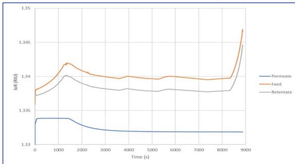
The ability of the mPath IoR sensor to differentiate between different buffer compositions allowed to obtain deeper process insight. The signal obtained from the permeate stream allows for characterization of the process buffer matrix in real time. During diafiltration this can be used to assess the progression of buffer exchange. The mPath IoR sensor permeate stream signal during diafiltration is seen in Figure 4.
