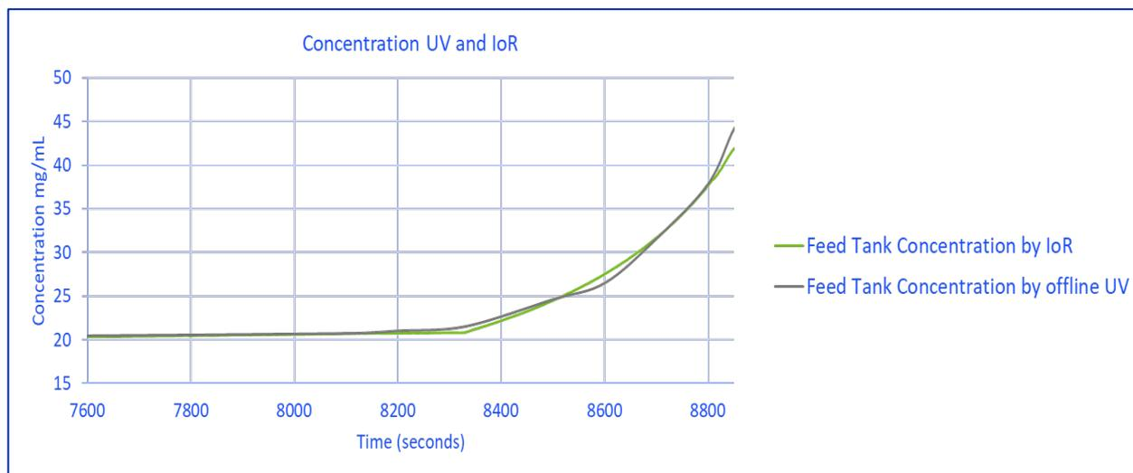
The process concentration calculations utilizing the mPath IoR sensors are shown to accurately track the offline measurements by UV. Even at high concentration levels seen during the second ultrafiltration, measurements obtained with the use of the mPath IoR sensor are highly accurate. This method eliminates the need for offline concentration measurements and subsequent dilution procedures to achieve the desired concentration.
