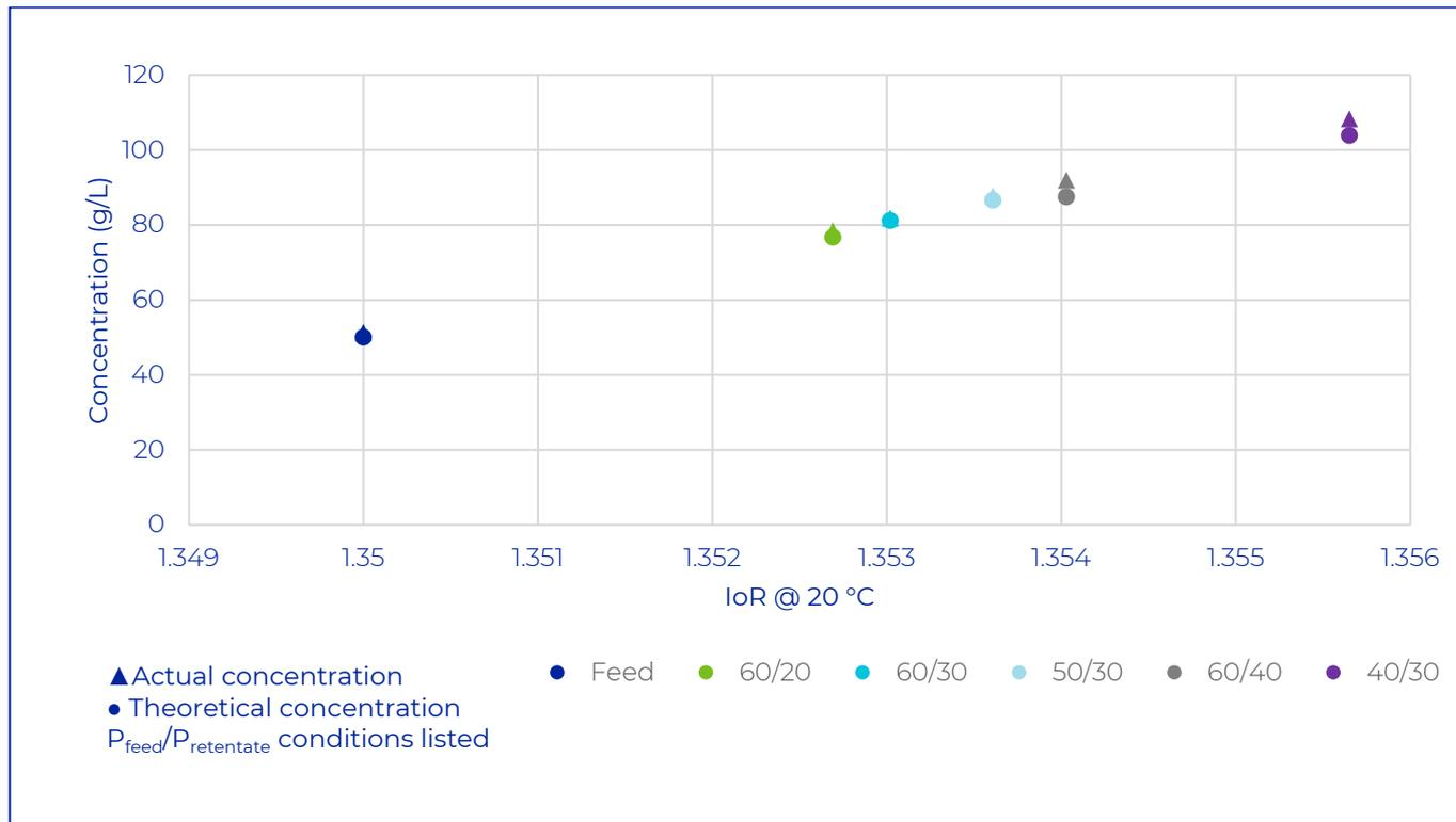
It is shown from the data in Figure 6 that the mPath IoR is a useful tool for process characterization. A strong correlation between the actual and theoretical concentration values is shown, with less than five percent difference across six distinct measurements. When establishing the highest concentrations that can be achieved with a given configuration, the mPath IoR can replace the need for offline sampling. This reduces time and resources needed for process optimization.
