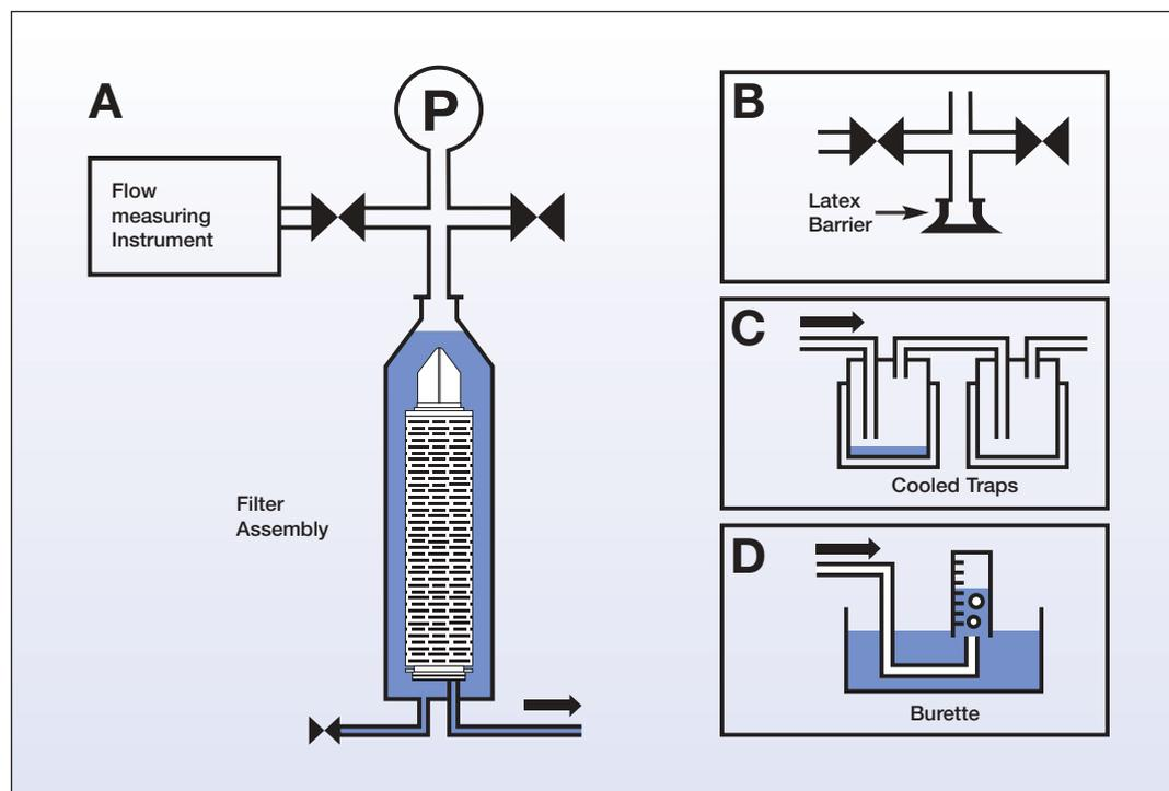
**Figure 1:** System for performing the Water Intrusion Test
