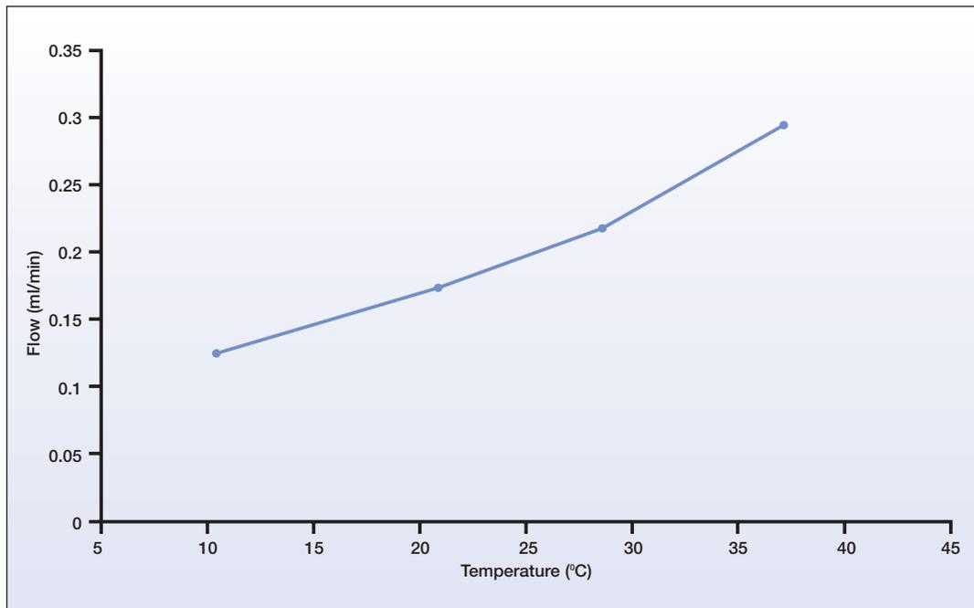
*Figure 4: Flow rate as a function of temperature*
