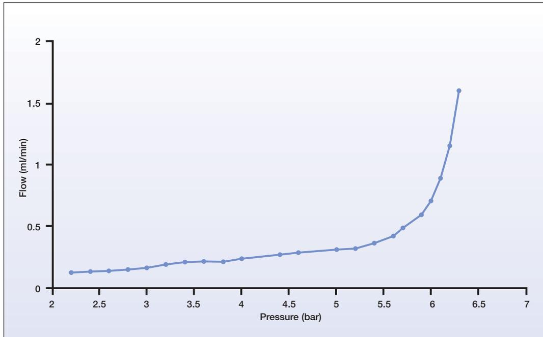
*Figure 2: Flow rate as a function of pressure*
