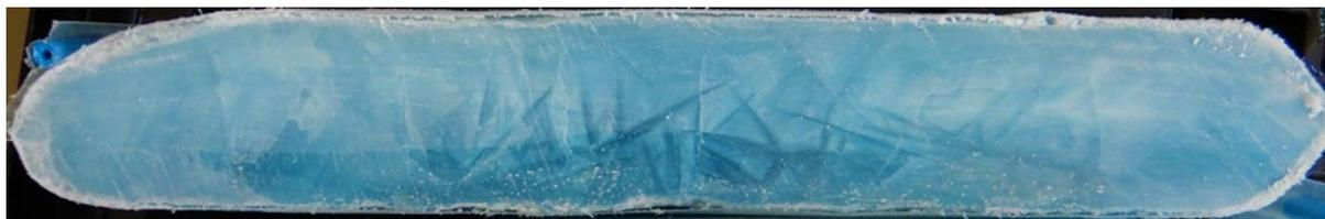
B. Plate freezer 'fast freezing' - Homogenous freezing (no dark spots) indicating cryoconcentration is significantly reduced
