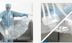
Confirm tubing on inlet and outlet ports is securely connected
