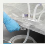
Slide the Allegro biocontainer into the tote and align the locating plate in the cutaway in the bottom of the tote
