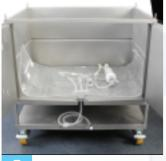
Ensure side panels of the Allegro biocontainer are facing upwards, with tubing and components connected to the top ports placed in the center of the folded biocontainers
