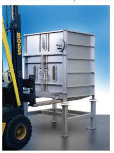
4. Ensure the base modules feet are completely aligned with the holes on the stand frame so the bolts can be inserted (Figure 4).
