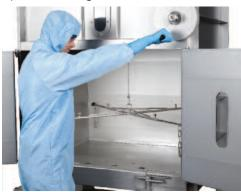
9. Prior to Allegro biocontainer installation, the lift pin needs to be released to unlock the port plate clamp (Figure 18).
