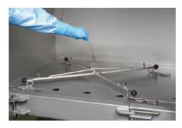
7. To extend the cross frame arms, turn the knob on each arm and slide each arm to the four tote corners. The cross frame arms should be adjusted so they are 15 – 20 mm from the tote inner corners (Figure 16).
