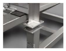
5. Once the bolts on the base module are aligned with the holes on the stand, slowly lower the fork lift to drop the bolts into place (Figure 5).
