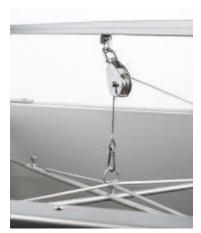
2. Feed the stainless cable through the pulley on the top corner of the extension module and pull the cable toward the ground until the carabiner rests on the pulley (Figure 12).
