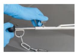
8. Using the friction wheel, raise the crossbar inside the tote to prepare for biocontainer installation (Figure 17).
