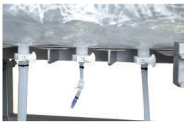
6. Close all clamps on the outlet lines and ensure that the inlet lines are open on the biocontainer. Secure the lower swivel door and replace locking pin. Attach the four hoist clips to the holes four holes located at each corner of the top of the biocontainer. Ensure each clip fastens to the corresponding hole so that the crossbar is holding the four connection points (Figure 22).
