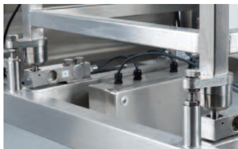
Nuts in the raised position for transportation
