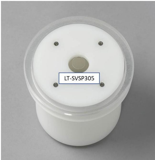
Figure 12 - Magnetic clamp assembled with centering aligner.
