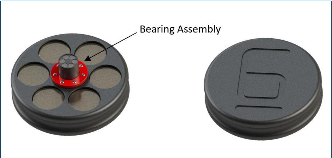
Figure 29 - Four magnet charger (LT-SVSP306). During the charging procedure, ensure that the ball bearing assembly is fully resting on the surface of the levitation drive head.
