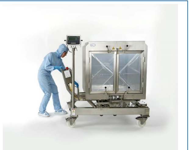
Figure 24 – Lift drive unit and latch to tank.
