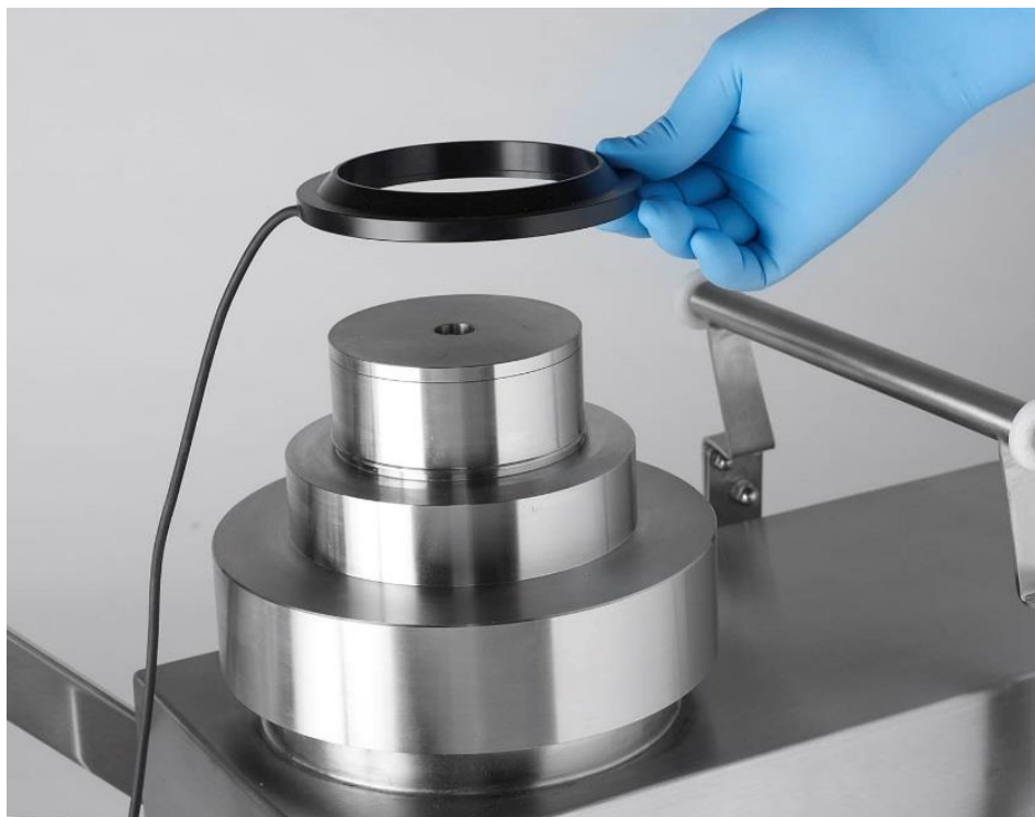
Figure 48 – Sensor ring replacement.
