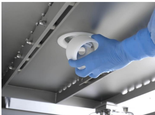
Figure 21 – Removal of magnetic clamp.
