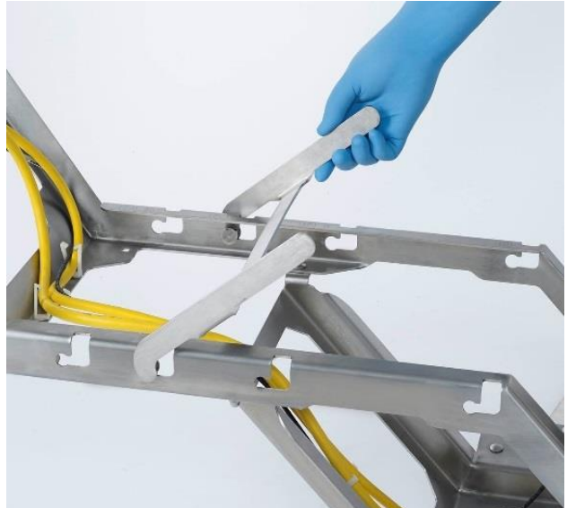
2. Rotate the latch clockwise until the axle flats are aligned with the horizontal slots.
