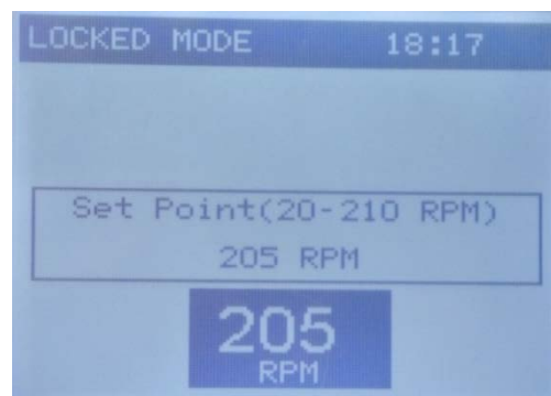
Figure 32: Local speed control in locked mode
