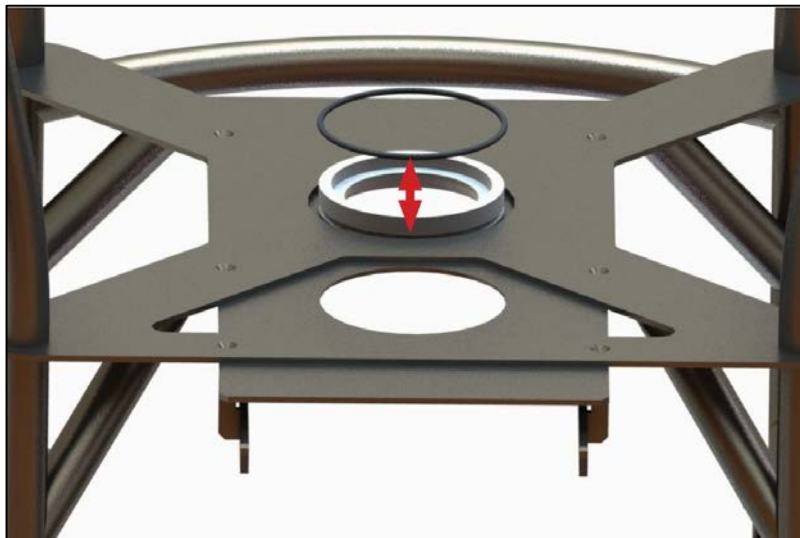
Figure 8: Installation of the drive-biocontainer interface on tank dolly with o-ring
