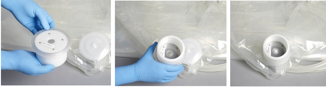
Figure 15 : Assembly of Allegro mixing biocontainer with magnetic clamp/aligner assembly
