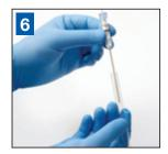
Prior to placing the Allegro singleuse needle into the filling machine, hold the needle by the hub and remove the protective sheath.
