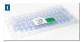
Remove the bag from the box in a clean area, do not remove inner bags until you are inside a clean room.
