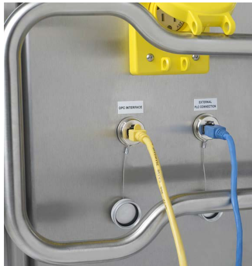
Figure 5.5 Ethernet ports (OPC Interface and External PLC Connection)
