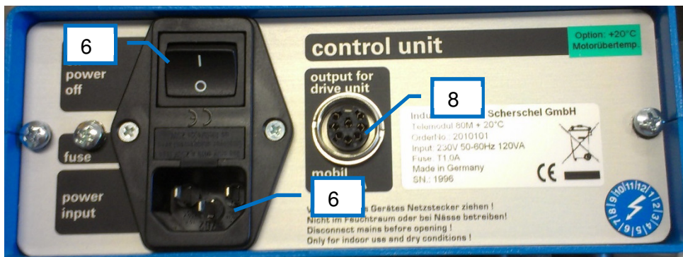
Figure 6: Back of control unit
