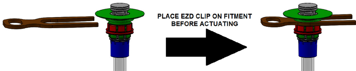
Figure 17: EZ Drain clip installation
