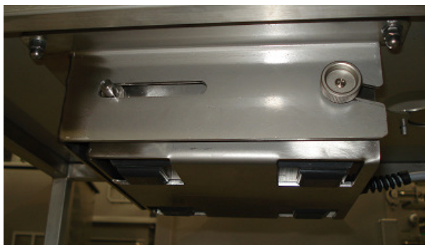
Figure 12: Correctly installed drive unit in final position
