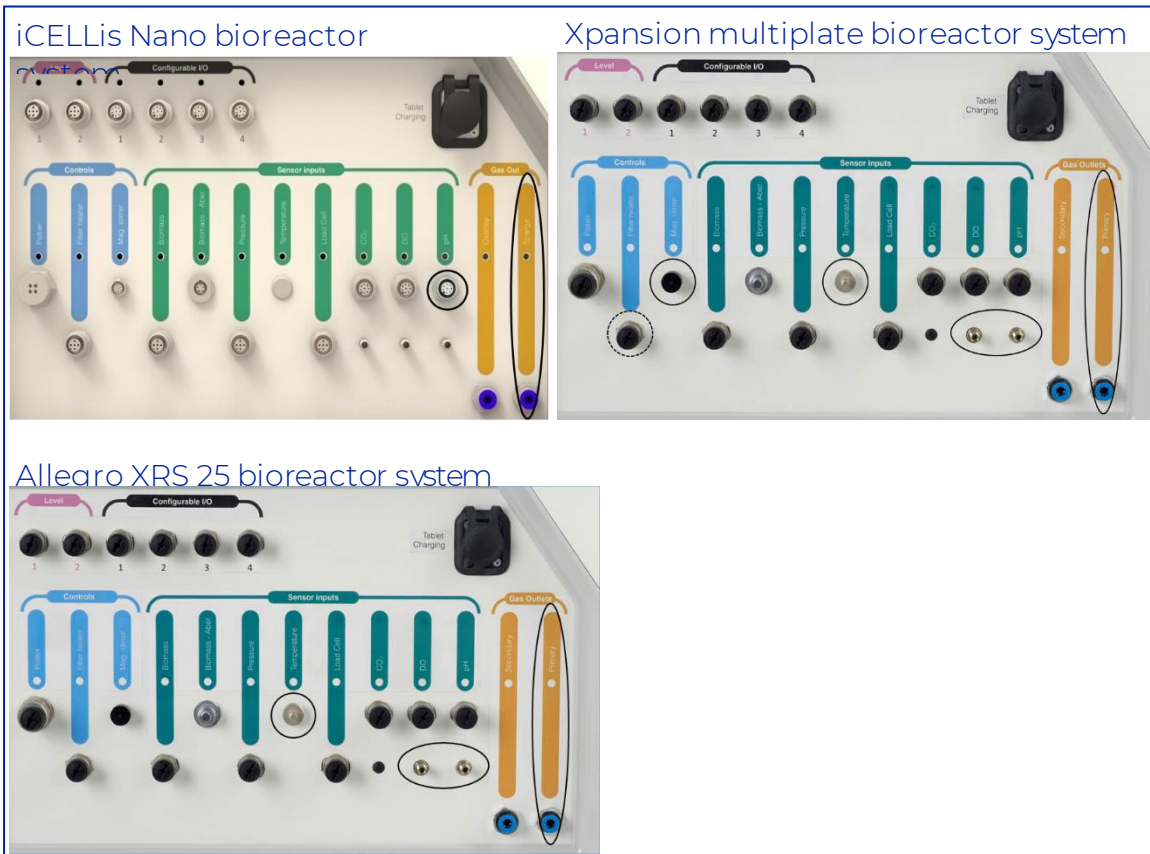
Figure 10 Side panel connections.
