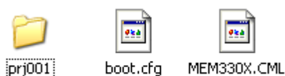
Figure 47: Overview of files and folders to be saved on the CF card
