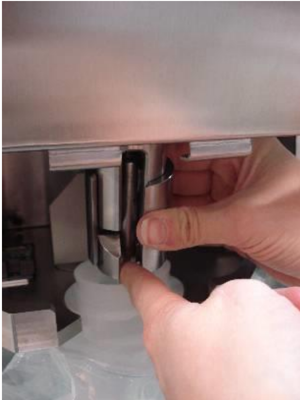
Figure 38: Inserting the mixing stick in the connection cylinder and closing the cylinder
