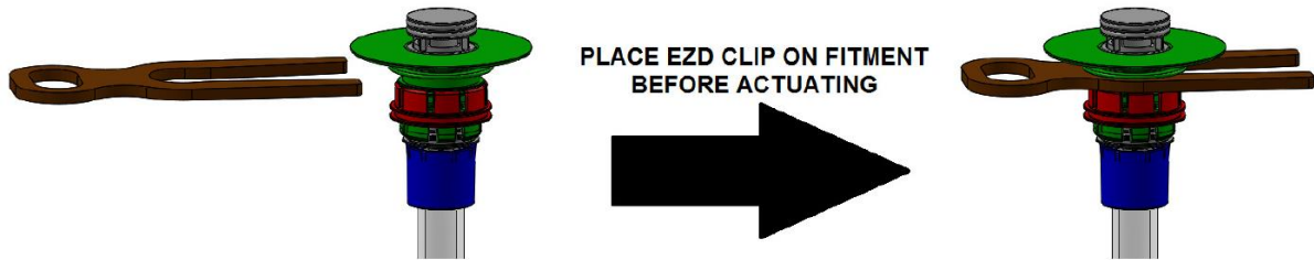
Figure 27: EZ Drain clip installation
