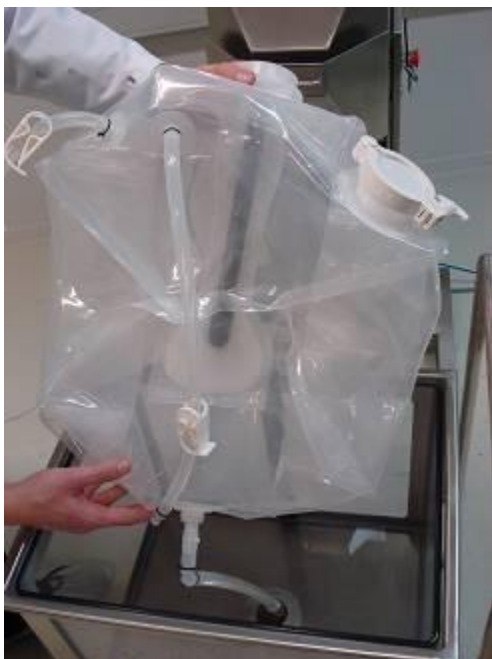
Figure 26: Installation of a 50L PadMixer biocontainer in the mixing tank
