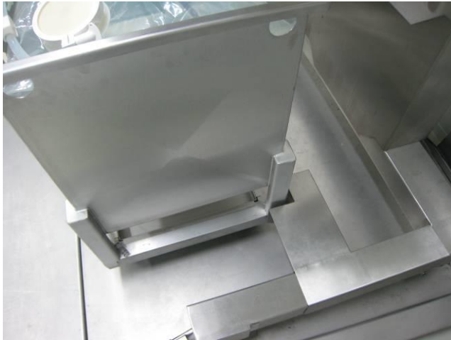
Figure 34: Positioning 200L mixing tank
