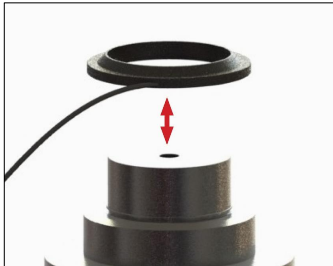
Figure 28: Sensor ring replacement
