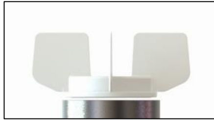
Figure 11: Test impeller levitates above the head of the super-conductive drive unit during a levitation test.
