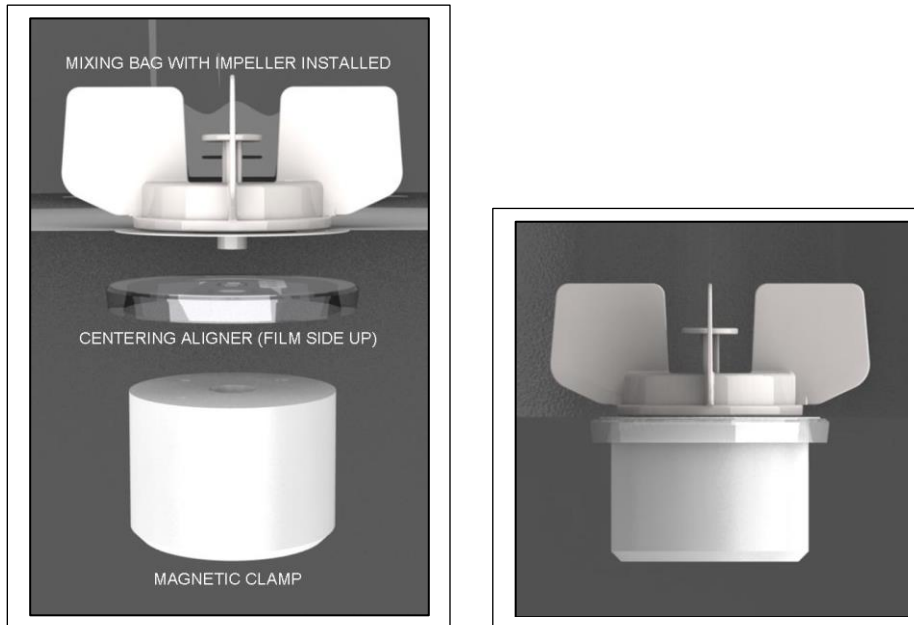
Figure 17: Assembly of dry bag with interface
