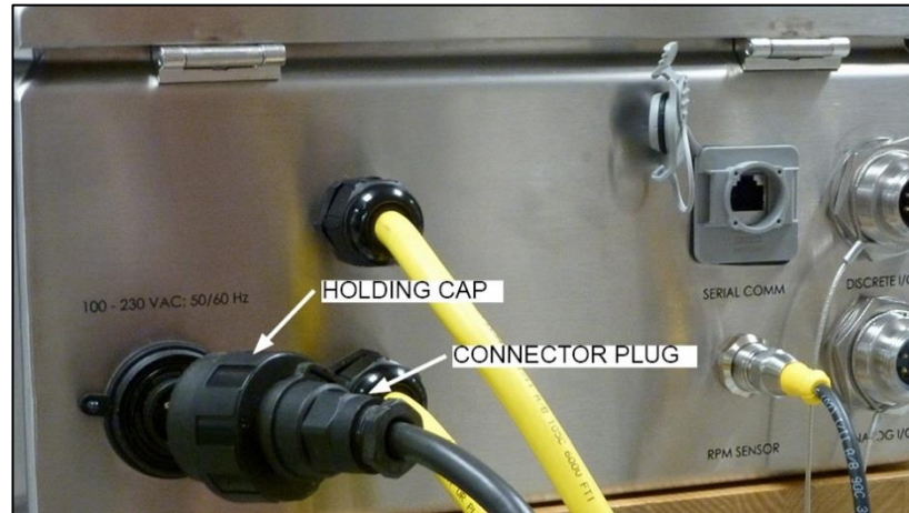
Figure 29: Power cord replacement
