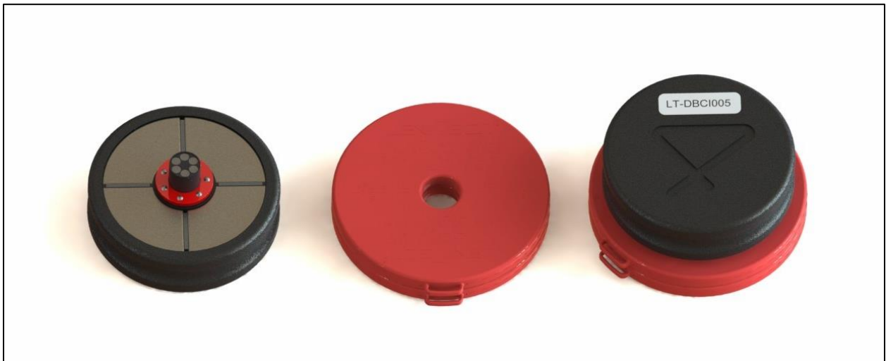
Figure 4: From left to right, Magnetic Charger (DBCI005), Shield for Magnetic Charger, (DBAK011) and Magnetic Charger (DBCI005) coupled with Shield. During the charging procedure, the ball bearing (red in far left picture) should rest on the surface of the levitation head of the drive unit.
