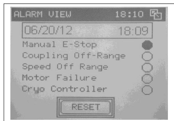
Figure 56: Failure detection screen
