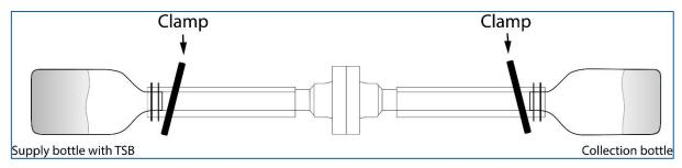
Assembly connected by Kleenpak Presto sterile connector for transfer of TSB
