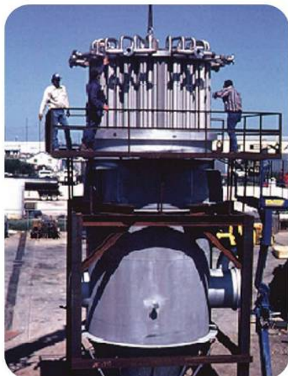
Fig. 2 — Typical coal-gasification filter system illustrating tube sheet bundles consisting of hundreds of iron-aluminide porous tubes being lowered into their housings (top). A high-temperature gas feed stream laden with ash initially enters the housing and contacts the outside surfaces of the filter tubes. Filtered ash falls to the bottom of the vessel (bottom) where it is transported out of the system. Clean, hot gas that is filtered through the system is directed to a common outlet pipe and sent to the turbine inlet for power generation.
