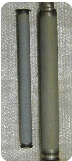
Fig. 1 — Iron-aluminide single element filter (2 in. diameter by 20 in. long) and an internal fuse.
