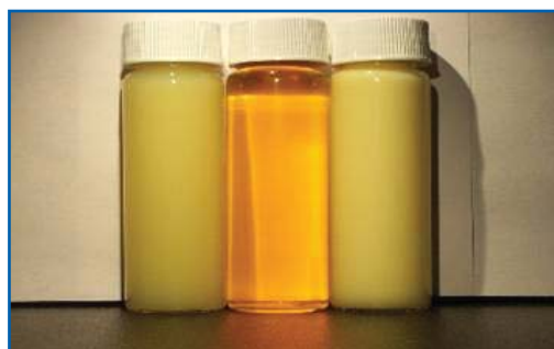
Fig 2: Emulsion on (left), BioDiesel exiting coalescer (middle), acid water phase collected from coalescer (right)
