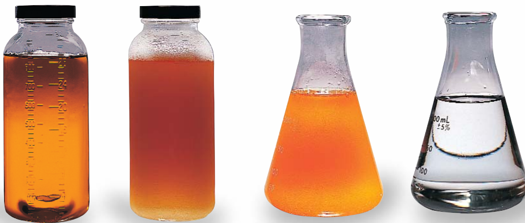
Pall's AquaSep Plus and PhaseSep liquid/liquid coalescers separate water from hazy diesel and oil from wastewater, providing contaminant-free products.
