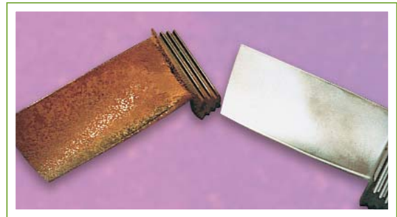
Left: Deposits form on a turbine blade. Right: A turbine blade protected by a SepraSol liquid/gas coalescer.
