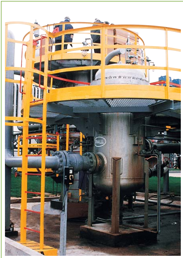
Vertical AquaSep Plus liquid/liquid coalescer system removing water from diesel.
