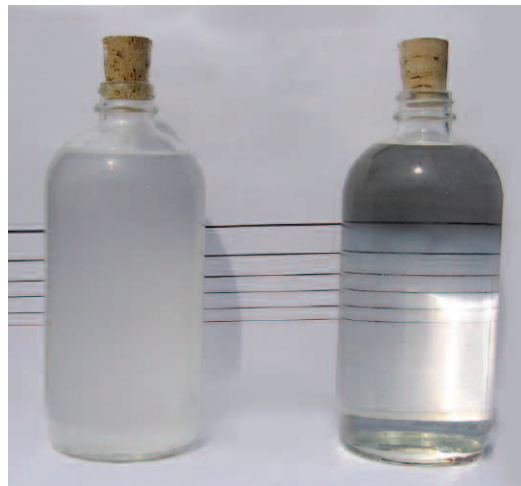
Figure 1: Liquid/Liquid coalescer influent (~600 ppmv total water) on left. "Clear & Bright" coalescer effluent on right.
