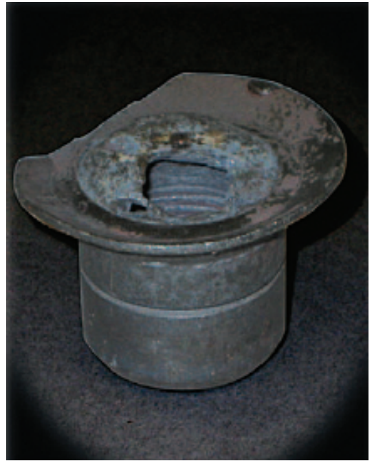
A fouled burner tip
